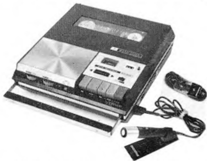
Automatic track reversal is a feature of this Standard mains/battery portable
